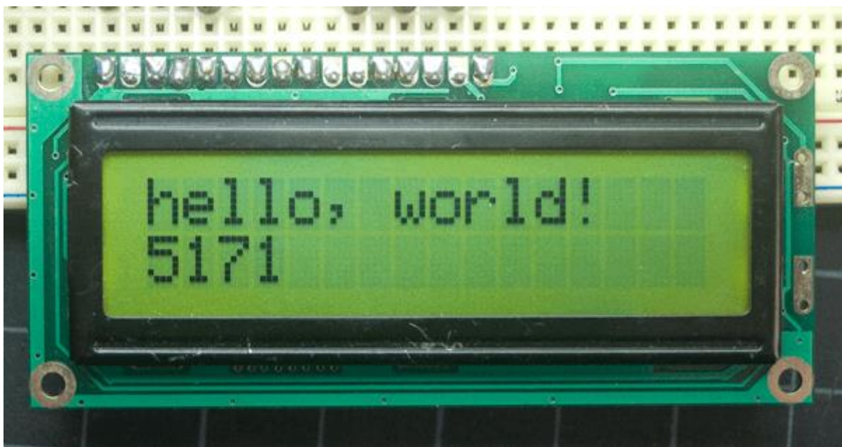
Fig. 21 Output of the sketch in 16x2 LCD
